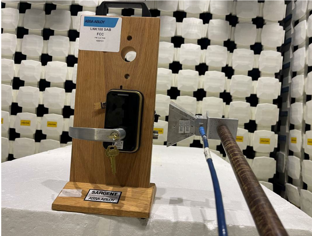
Test Setup, RE 18-25 GHz
