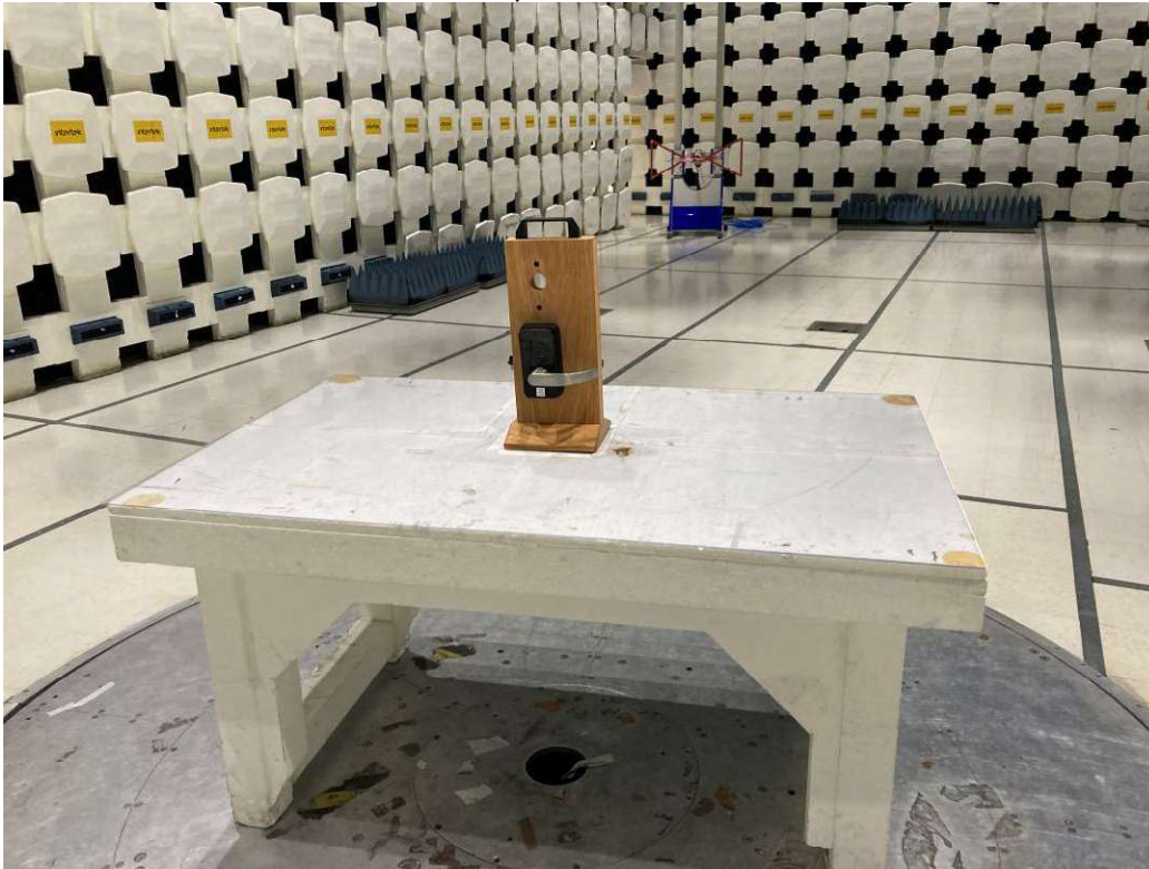
Test Setup, RE 30-1000 MHz
