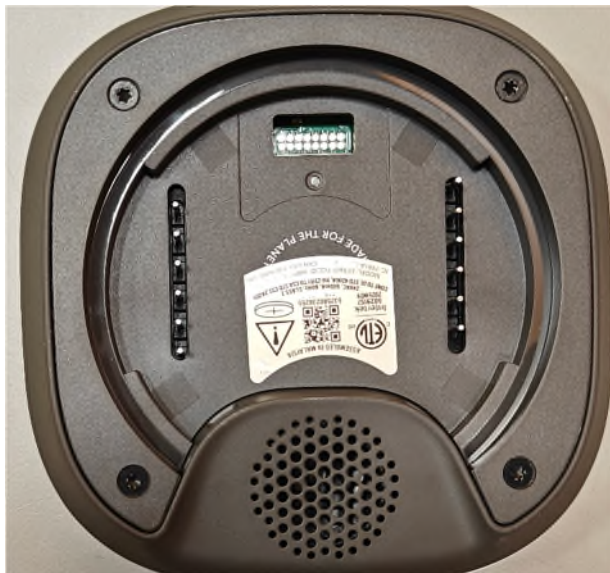
Figure 3 – ECB601: Back view with I/O ports
