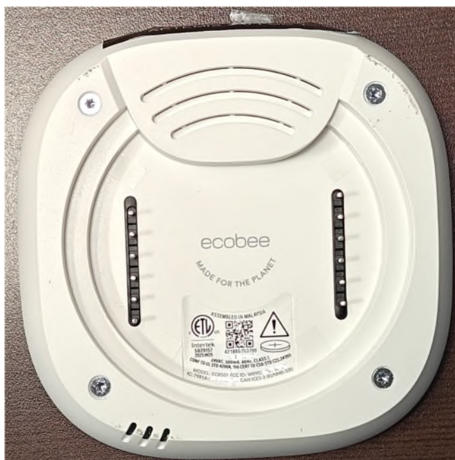
Figure 3 – ECB501: Back view with I/O ports
