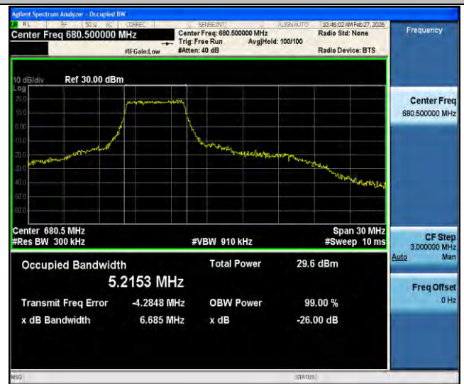
Band71-15MHz-16QAM-133297-27RB#0-PASS
