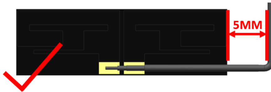
FIGURE 5.2.1 RECOMMENDED CABLE BENDING RANGE
