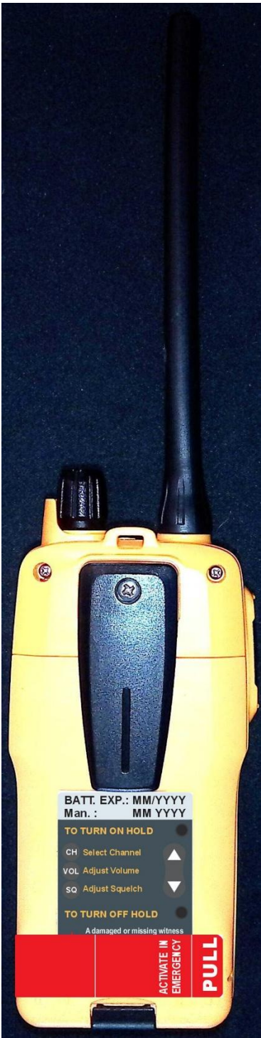
Figure 4: safeSEA V200 Rear View with Battery & Witness Label
