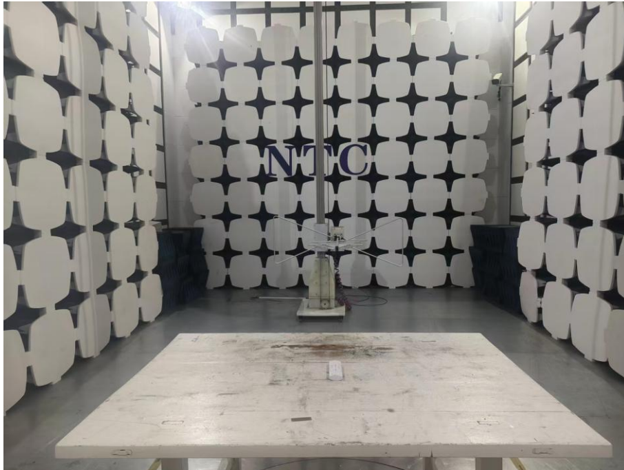
Photos of radiated emission test Above 1GHz
