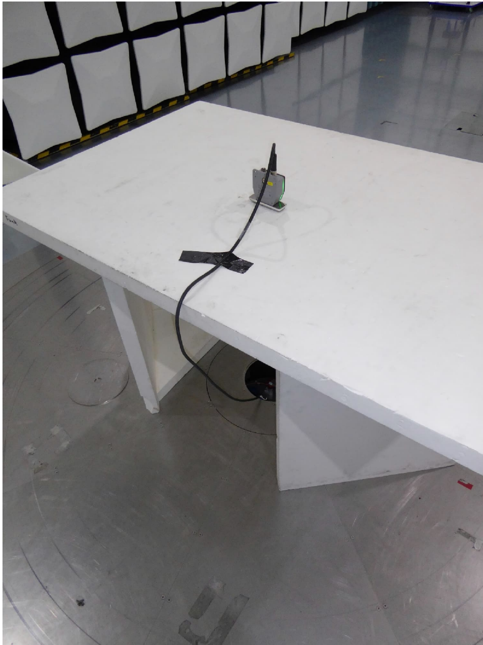
Test setup semi anechoic chamber (position 1)
