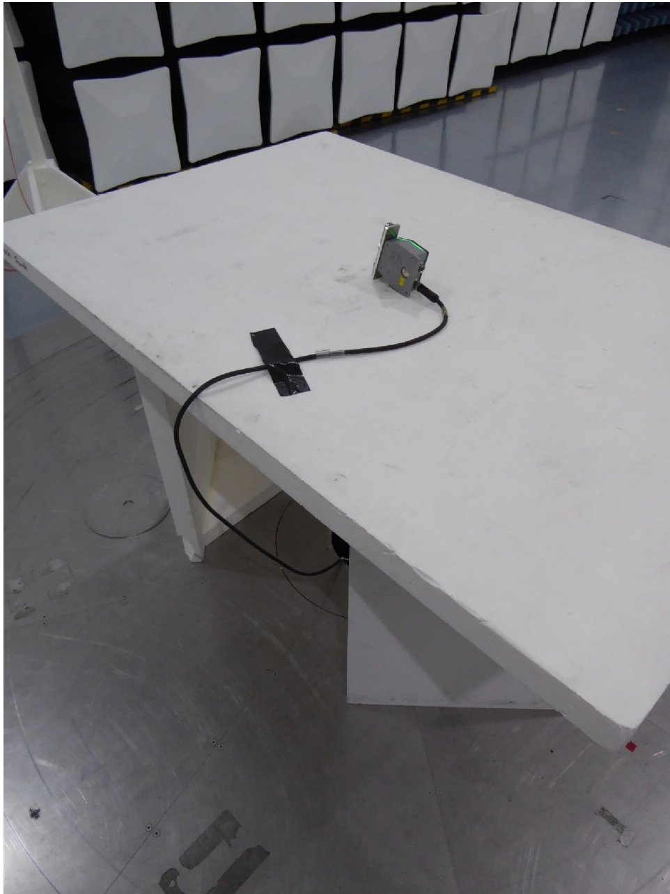
Test setup semi anechoic chamber (position 2)
