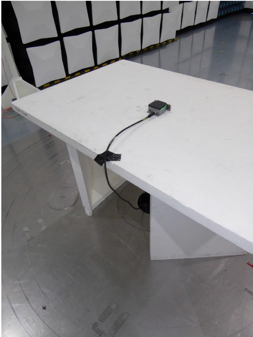
Test setup semi anechoic chamber (position 3)
