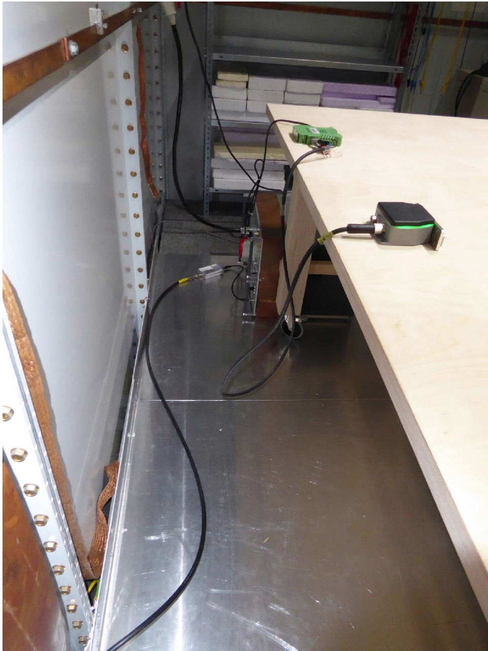
Test AC power line conducted emissions
