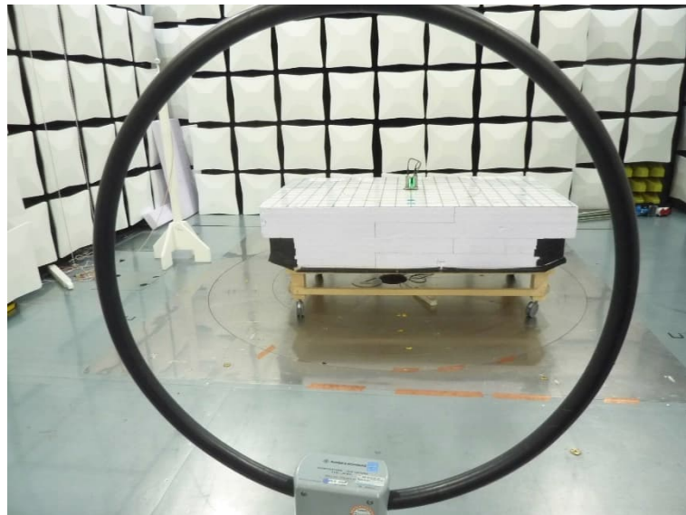
Test setup semi anechoic chamber <30 MHz
