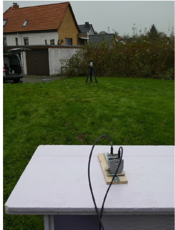
Test setup outdoor test side <30 MHz
