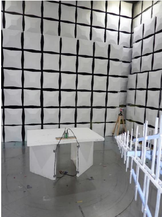
Test setup semi anechoic chamber <1 GHz
