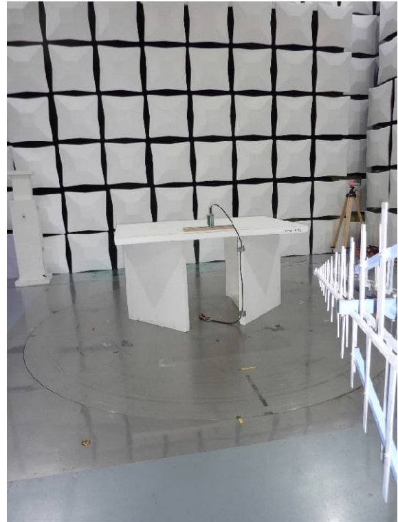
Test setup semi anechoic chamber <1 GHz
