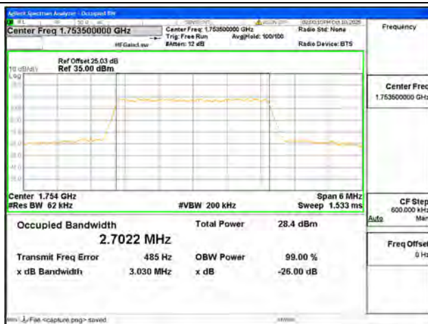
B4 / 3MHz / 16QAM/ High CH
