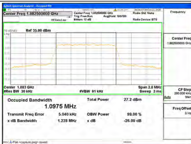
B25 / 1.4MHz / 16QAM/ Mid CH
