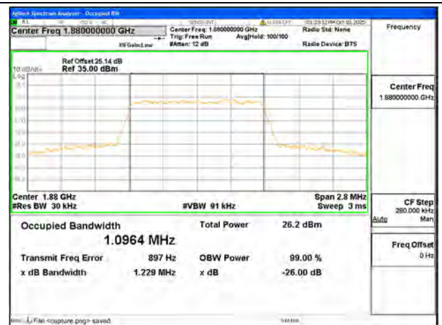
B2 / 1.4MHz / 64QAM/ Mid CH
