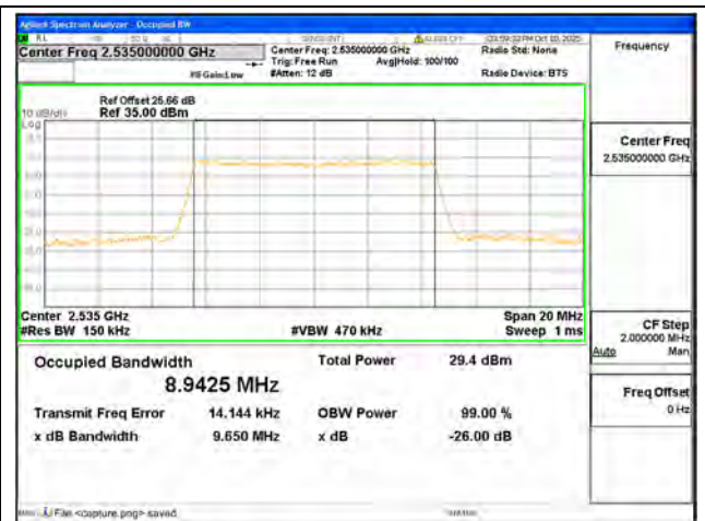
B7 / 10MHz / 16QAM/ Mid CH
