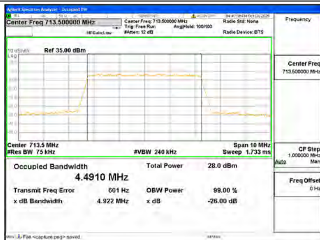
B12 / 5MHz / 64QAM/ High CH
