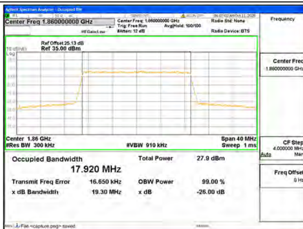
B25 / 20MHz / 16QAM/ Low CH
