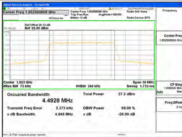
B2 / 5MHz / 64QAM/ Low CH
