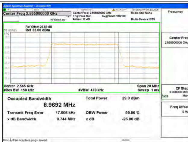
B7 / 10MHz / 16QAM/ High CH
