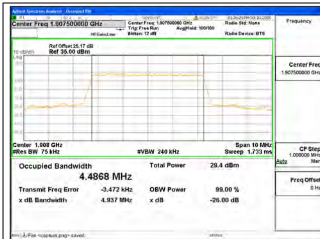
B2 / 5MHz / QPSK/ High CH
