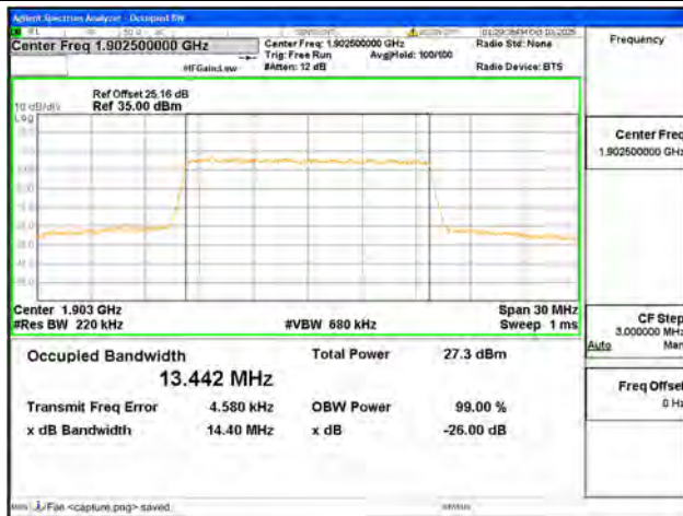
B2 / 15MHz / 64QAM/ High CH
