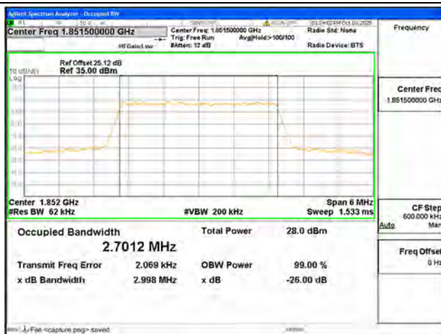
B2 / 3MHz / 16QAM/ Low CH
