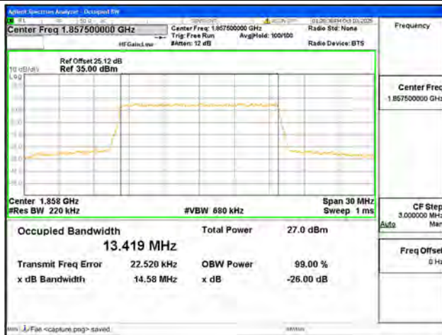
B2 / 15MHz / 64QAM/ Low CH
