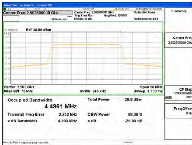
B7 / 5MHz / 64QAM/ Low CH
