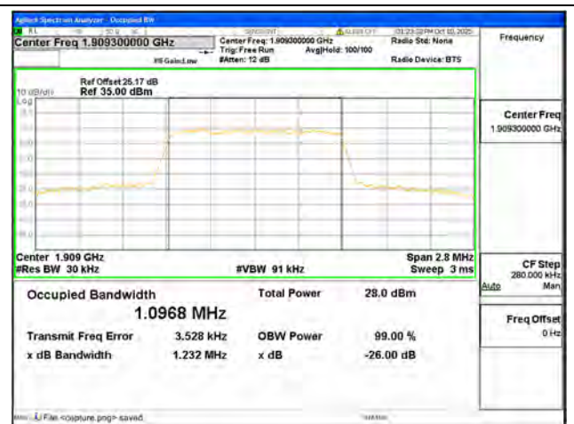
B2 / 1.4MHz / 16QAM/ High CH
