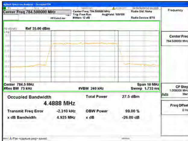
B13 / 5MHz / 64QAM/ High CH
