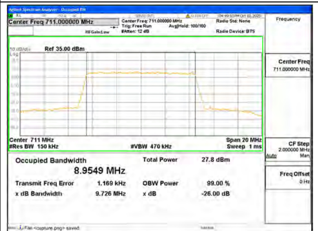
B12 / 10MHz / 64QAM/ High CH
