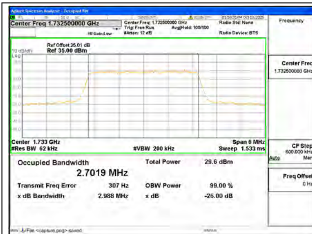
B4 / 3MHz / QPSK/ Mid CH
