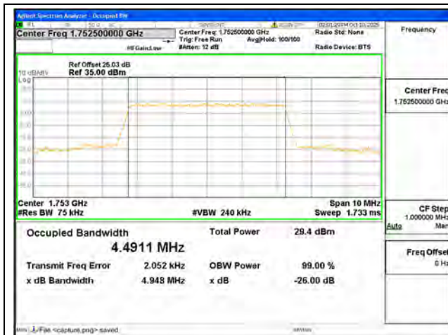
B4 / 5MHz / QPSK/ High CH
