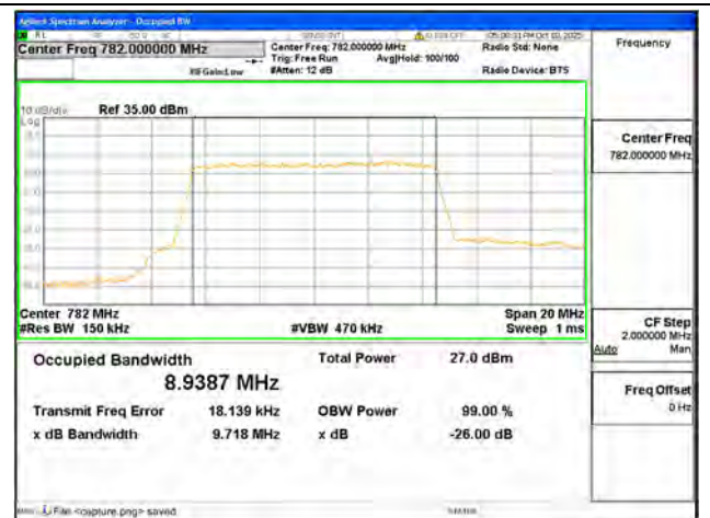
B13 / 10MHz / 64QAM/ Mid CH
