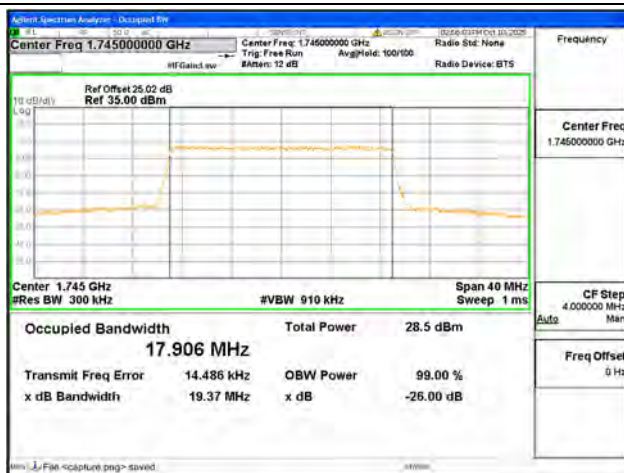
B4 / 20MHz / 16QAM/ High CH
