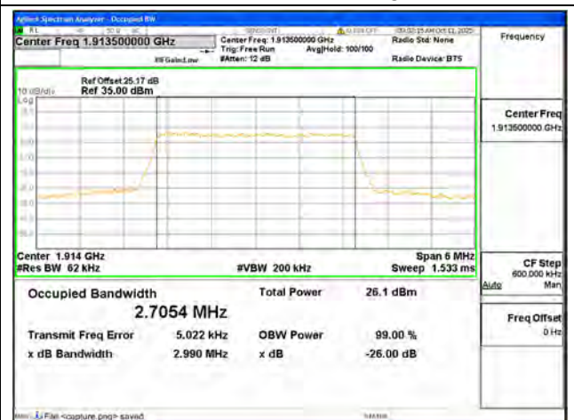
B25 / 3MHz / 64QAM/ High CH
