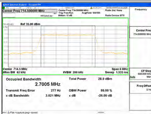
B12 / 3MHz / 16QAM/ High CH
