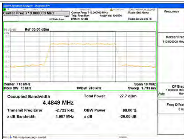
B17 / 5MHz / 16QAM/ Mid CH
