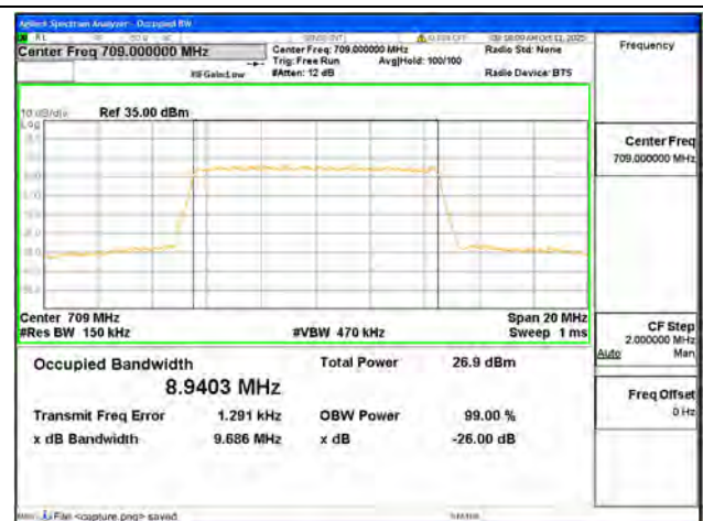
B17 / 10MHz / 64QAM/ Low CH
