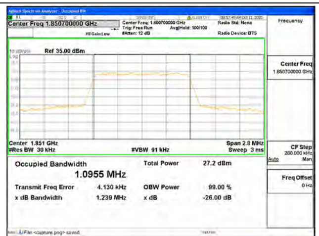
B25 / 1.4MHz / 16QAM/ Low CH
