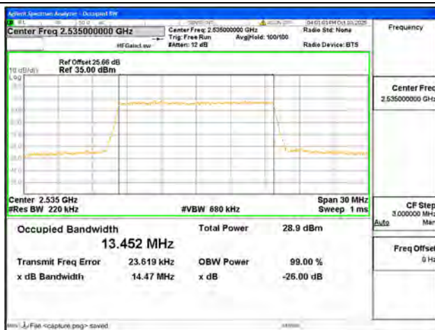
B7 / 15MHz / 16QAM/ Mid CH
