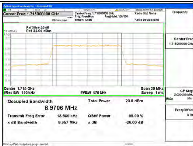
B4 / 10MHz / 16QAM/ Low CH
