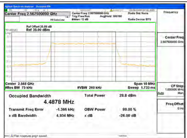
B7 / 5MHz / 16QAM/ High CH
