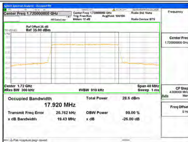
B4 / 20MHz / 16QAM/ Low CH
