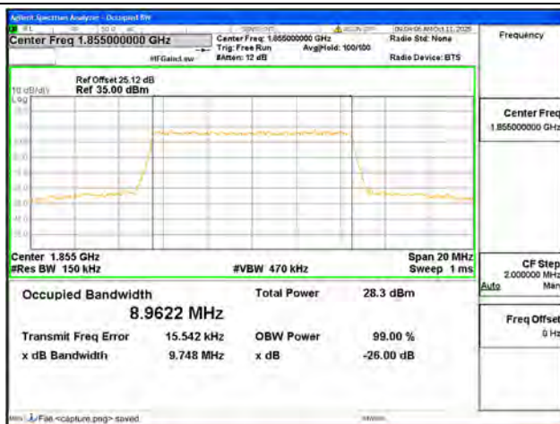
B25 / 10MHz / 16QAM/ Low CH
