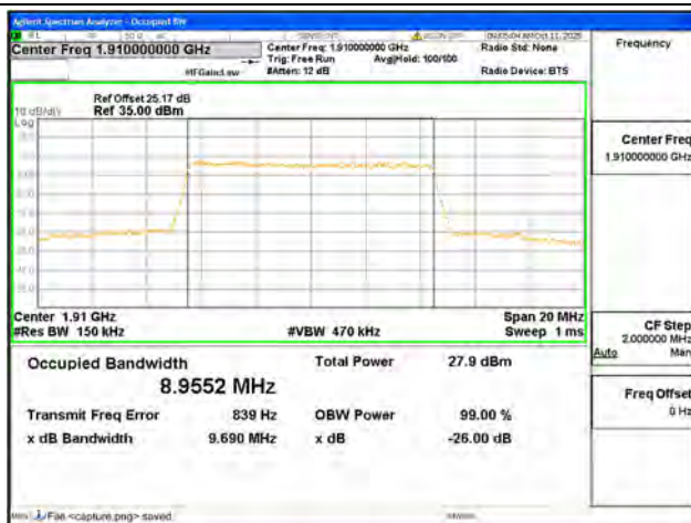
B25 / 10MHz / 16QAM/ High CH
