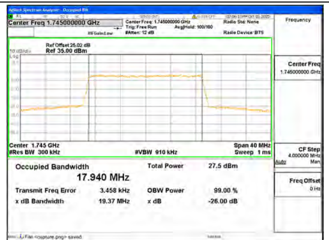
B4 / 20MHz / 64QAM/ High CH
