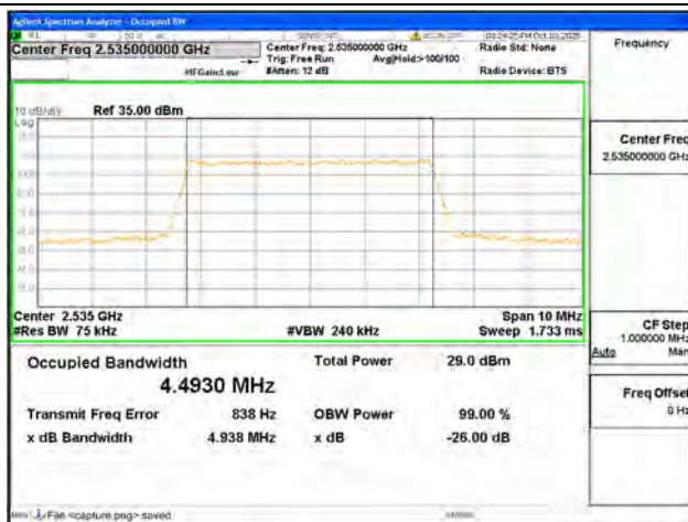
B7 / 5MHz / 16QAM/ Mid CH
