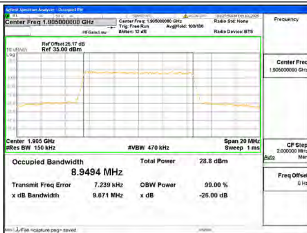
B2 / 10MHz / 16QAM/ High CH
