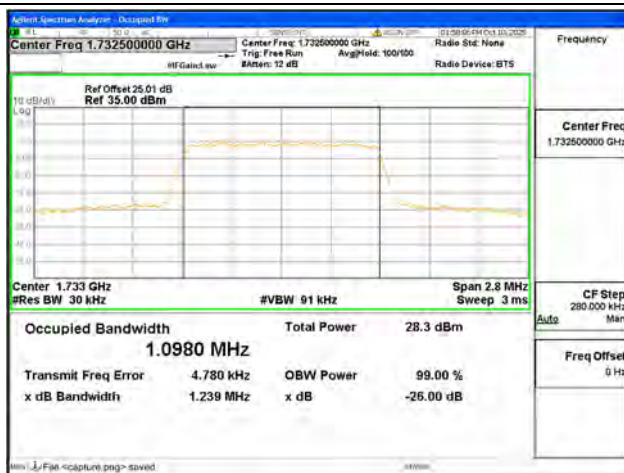
B4 / 1.4MHz / 16QAM / Mid CH
