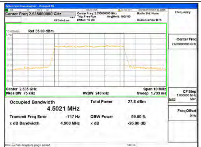
B7 / 5MHz / 64QAM/ Mid CH
