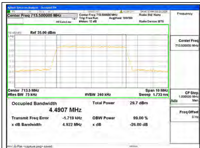
B12 / 5MHz / QPSK/ High CH
