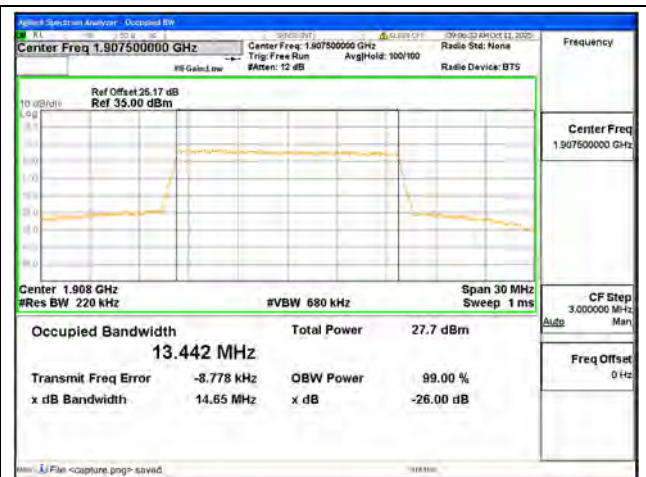
B25 / 15MHz / 16QAM/ High CH
