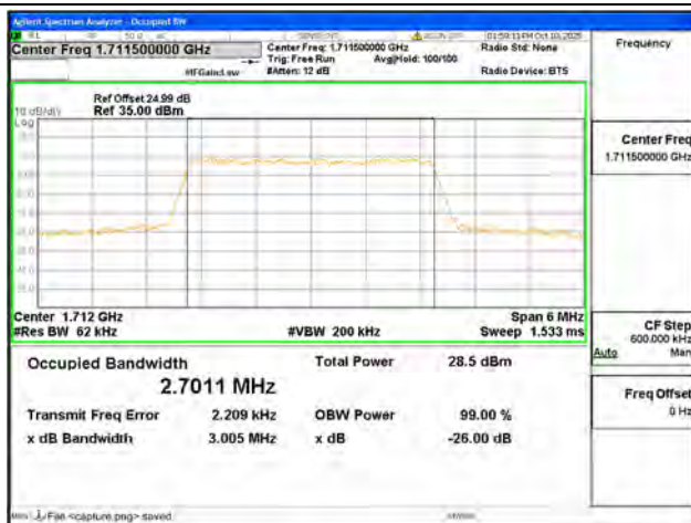
B4 / 3MHz / 16QAM/ Low CH
