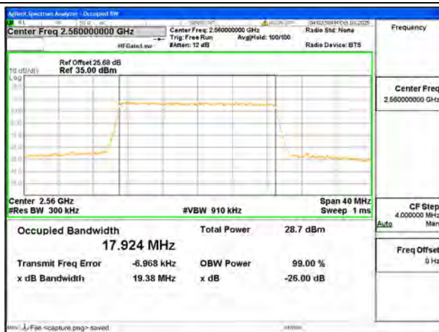
B7 / 20MHz / 16QAM/ High CH
