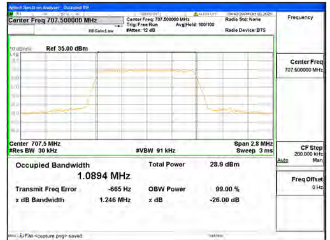
B12 / 1.4MHz / QPSK/ Mid CH
