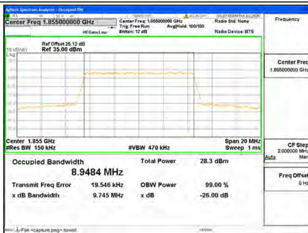
B2 / 10MHz / 16QAM/ Low CH
