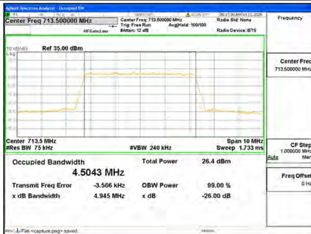
B17 / 5MHz / 64QAM/ High CH
