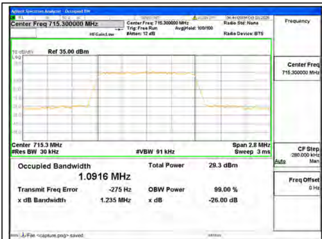
B12 / 1.4MHz / QPSK/ High CH
