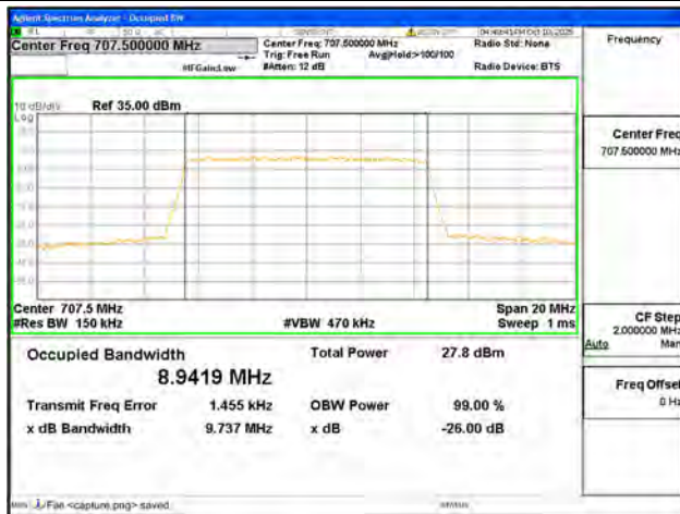
B12 / 10MHz / 64QAM/ Mid CH
