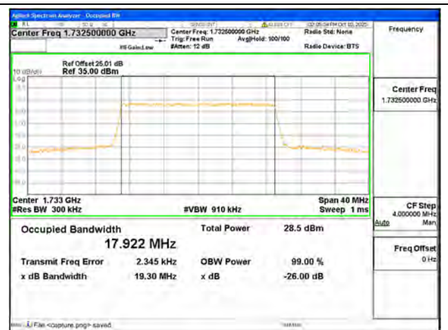
B4 / 20MHz / 16QAM/ Mid CH
