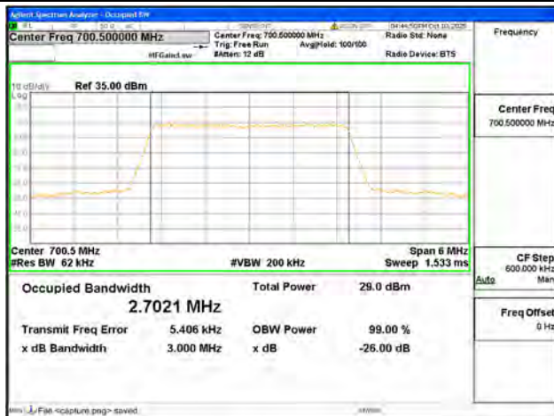
B12 / 3MHz / 16QAM/ Low CH
