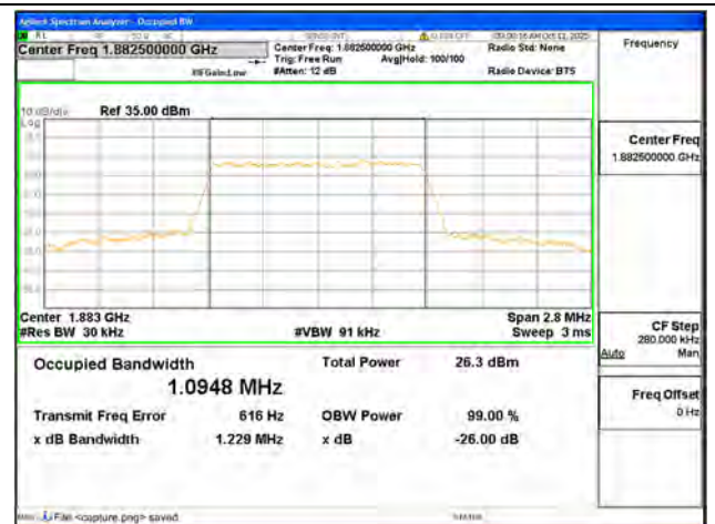
B25 / 1.4MHz / 64QAM/ Mid CH
