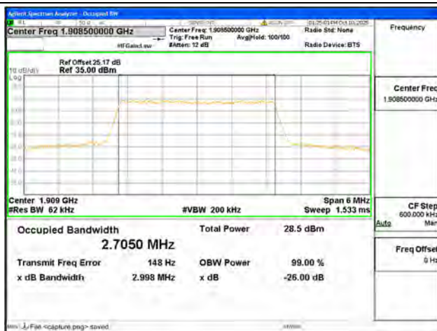
B2 / 3MHz / 16QAM/ High CH
