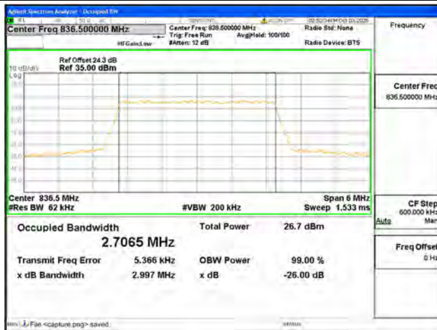
B5 / 3MHz / 64QAM/ Mid CH
