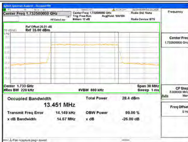
B4 / 15MHz / 16QAM/ Mid CH
