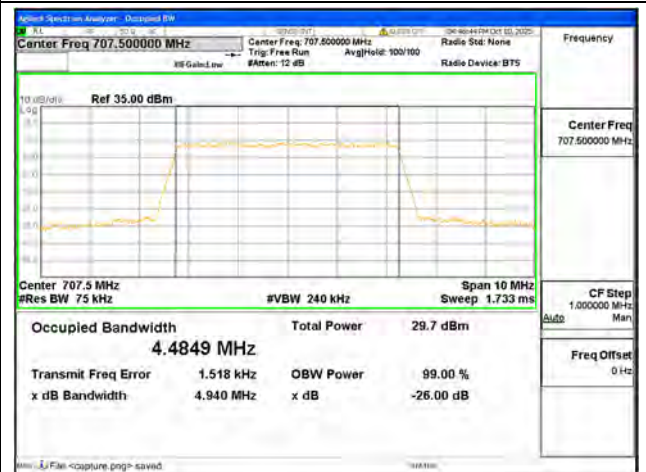
B12 / 5MHz / QPSK/ Mid CH
