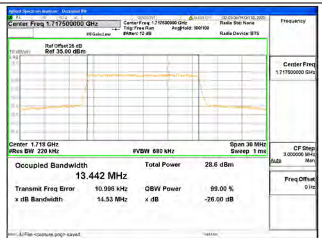
B4 / 15MHz / 16QAM/ Low CH
