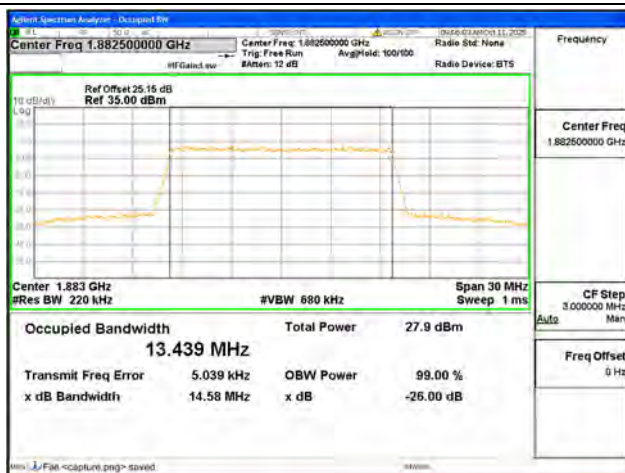
B25 / 15MHz / 16QAM/ Mid CH
