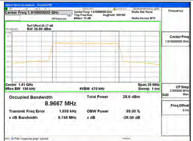
B25 / 10MHz / QPSK/ High CH
