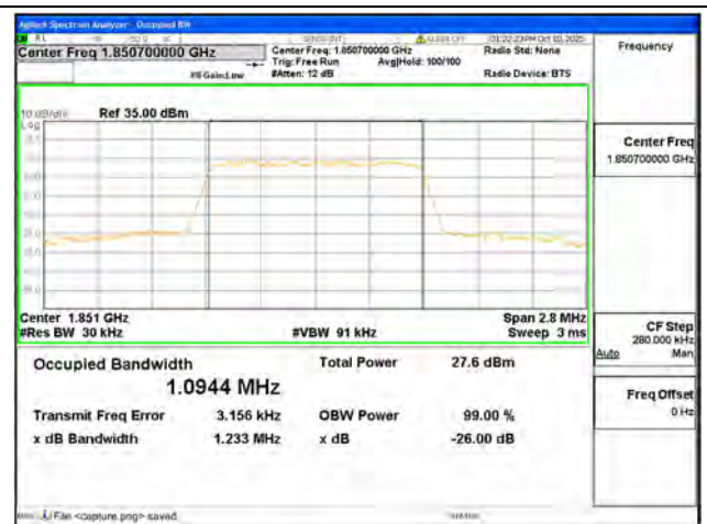
B2 / 1.4MHz / 16QAM/ Low CH
