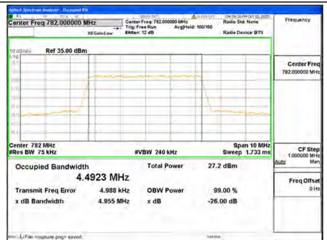
B13 / 5MHz / 64QAM/ Mid CH
