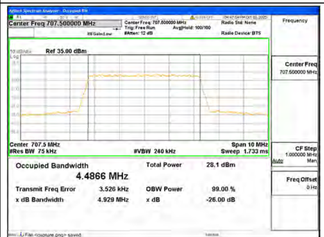
B12 / 5MHz / 64QAM/ Mid CH
