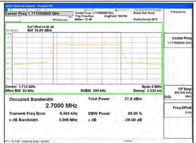
B4 / 3MHz / 64QAM/ Low CH
