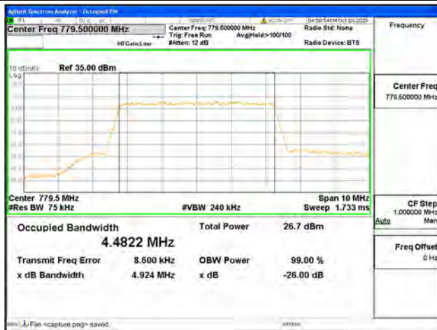
B13 / 5MHz / 64QAM/ Low CH
