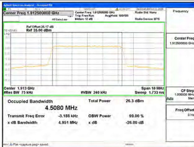
B25 / 5MHz / 64QAM/ High CH
