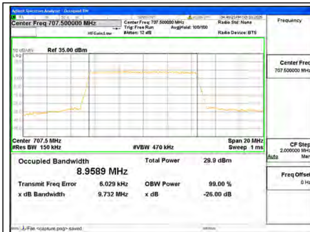
B12 / 10MHz / QPSK/ Mid CH
