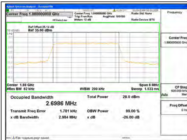
B2 / 3MHz / QPSK/ Mid CH
