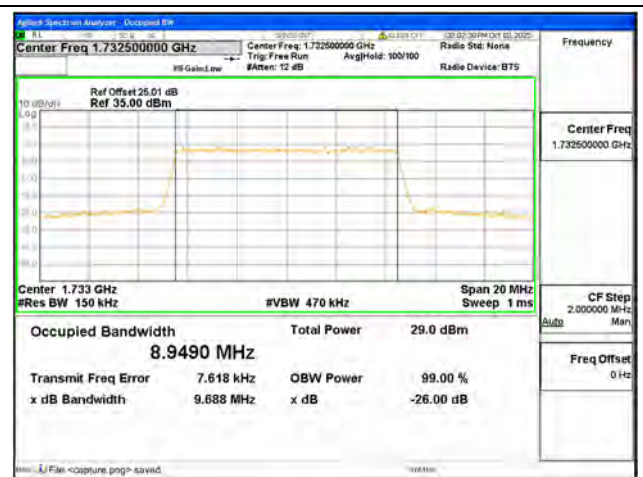
B4 / 10MHz / 16QAM/ Mid CH
