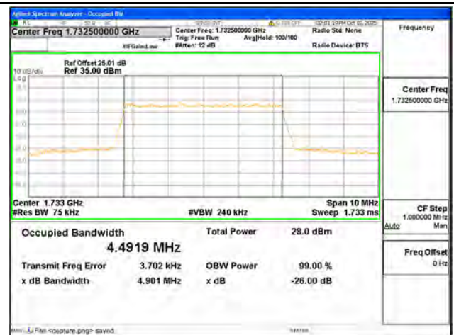
B4 / 5MHz / 64QAM/ Mid CH
