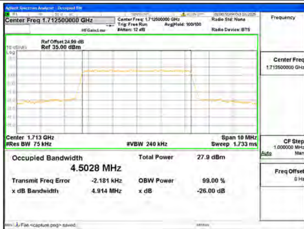
B4 / 5MHz / 64QAM/ Low CH
