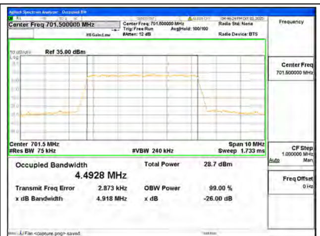
B12 / 5MHz / 16QAM/ Low CH
