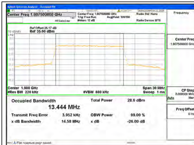
B25 / 15MHz / QPSK/ High CH
