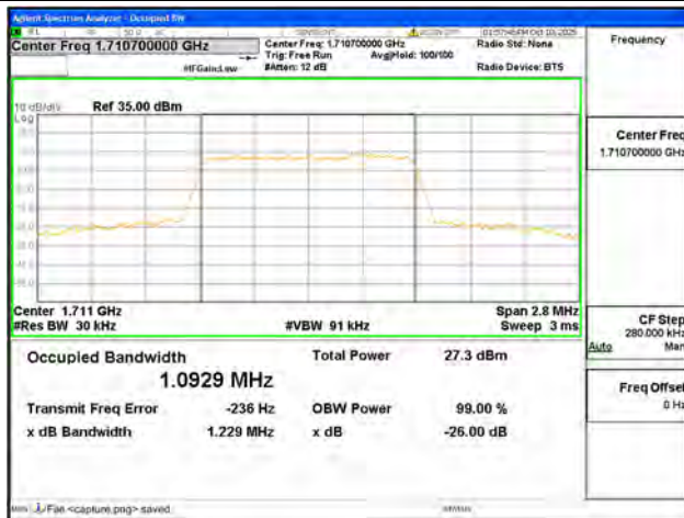
B4 / 1.4MHz / 64QAM / Low CH
