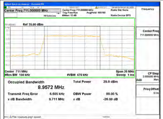
B12 / 10MHz / QPSK/ High CH
