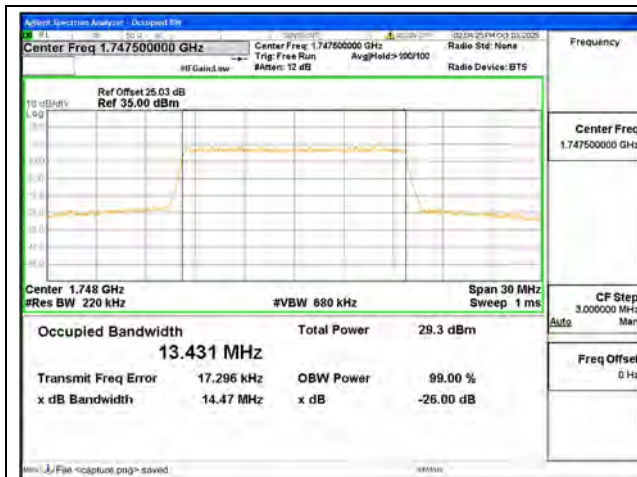
B4 / 15MHz / QPSK/ High CH
