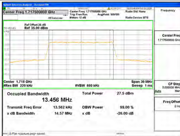
B4 / 15MHz / 64QAM/ Low CH
