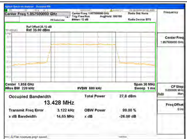
B2 / 15MHz / 16QAM/ Low CH
