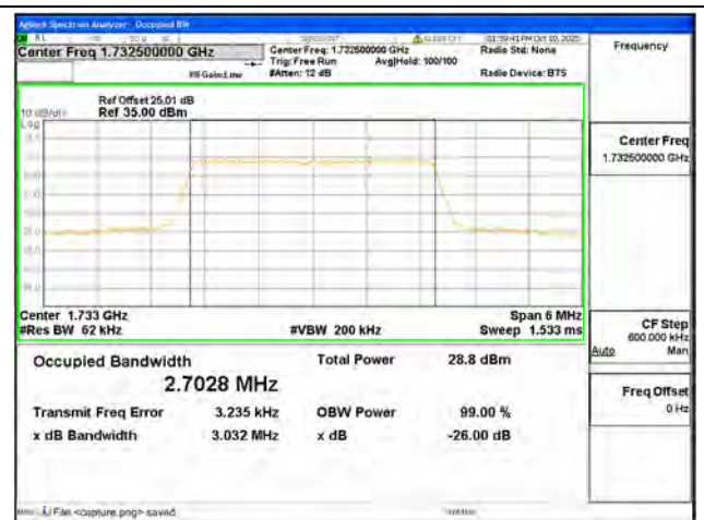
B4 / 3MHz / 16QAM/ Mid CH
