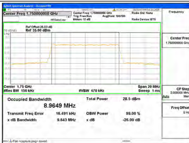
B4 / 10MHz / 16QAM/ High CH
